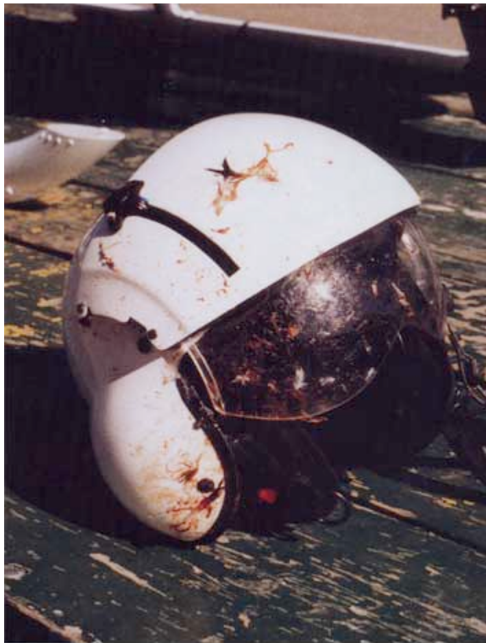
Plate 7 The helmet and face-shield probably saved the life of the pilot when he was struck in the face by windshield and bird debris. Photo courtesy Transport Canada.
