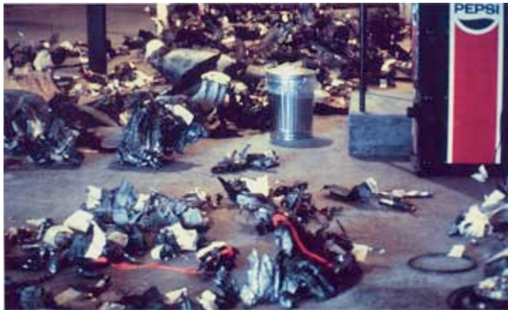
Plate 8 This is all that remains of a $200 million USAF B1-B bomber that crashed after striking an American White Pelican in Colorado. The airplane weighed 185,000 lbs, the bird 15 lbs. Three crew members died in the crash. Photo courtesy Transport Canada.
