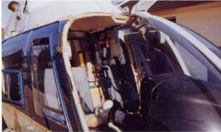
Plate 5 An impact with a Western Grebe (3 lbs) caused considerable damage to this helicopter. The bird struck the pilot in the face. Photo courtesy Transport Canada.
